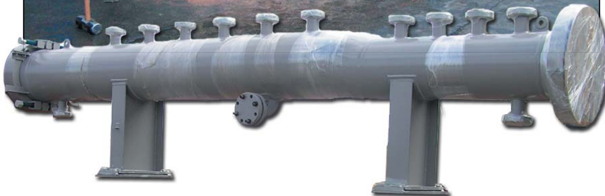
Pig Launcher ready for shipment.
